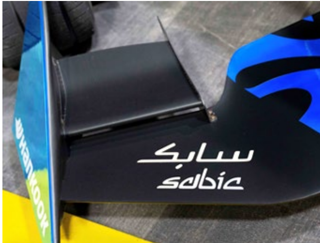
Materials such as front wing endplates (left), formed via a 3D printing process, and wheel fins (right) help reduce aerodynamic drag and enhance the race car's down-force stability.
