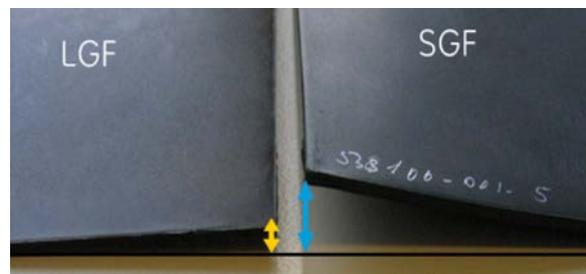
**Figure 2:** Picture is showing difference in dimensional stability between injection molded plaques of 30% PP SGF and STAMAX™ resin.
