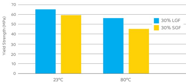
**Figure 3:** Graphic is showing difference in yield stress between 30% PP SGF and STAMAX™ resin according to Multiaxial Impact test at 23°C and 80°C.
