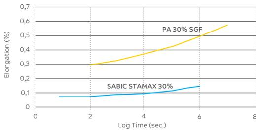
**Figure 1:** Graphic is showing creep performance of 30% STAMAX™ resin versus 30% SGF PA material.
