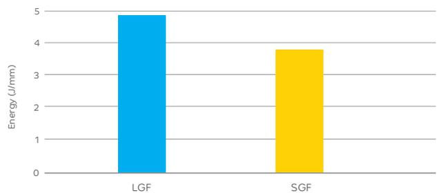
**Figure 4:** Graphic is showing difference in impact resistance between 30% PP SGF and STAMAX™ resin according to Multiaxial Impact test at 23°C.
